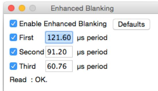
Enhanced Blanking is used to setup a special blanking which puts more power closer to the site at the sacrifice of range which is used to improve wave processing. Currently, Pulse Shaping needs to be disabled when enhanced blanking is enabled. Ask CODAR Support for more information on configuring Enhanced Blanking before trying this on your own.
