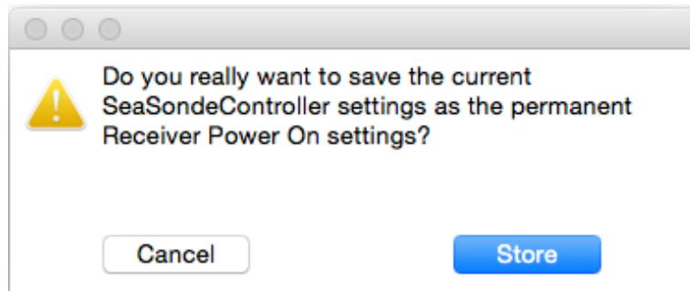
asks to permanently save the current settings as the receiver's or transponder's power up settings.
