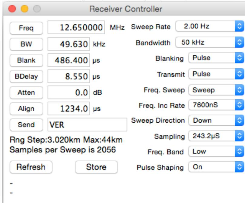
For normal operation and prevention of overdriving the transmitter and burning it out, you should **NEVER** set the BW to 0 (zero), or Freq. Sweep to **CW**, or **Transmit** to Full ON! These options are meant only for bench testing into a dummy load. If you accidentally do one of these settings, then you should quickly set it back to correct operation as the longer you leave it the more the amplifier will heat up and possibly be damaged.
