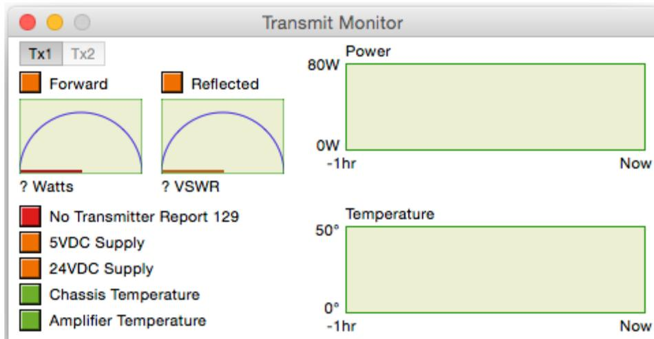
**No Transmitter Reports/Measurements OK** if red shows that the receiver was unable to communicate with the transmitter to obtain any information. This may be due to the transmitter being off, transmitter does not have the capability, or a hardware problem. It may also show red with bad measurement message, if there is a problem with the A/D converter hardware.
