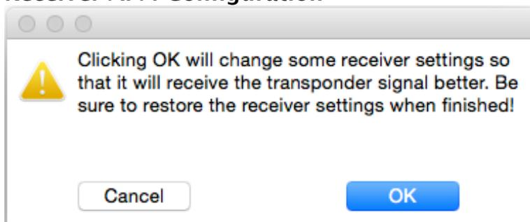
adjusts the receiver settings for use with transponder when measuring antenna patterns. When configuring the receiver and transponder together, you can use the Transponder control window Setup button to perform the same function.
