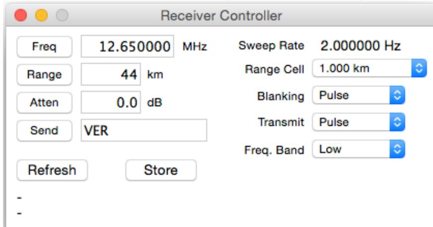
**Freq** is the center transmit frequency. Be careful not to set a frequency for which you do not have approval for. The band will automatically change depending on the entered frequency. If you enter a frequency outside the high or low band for your system the entry will automatically change to the lower or upper end of the closest band.
