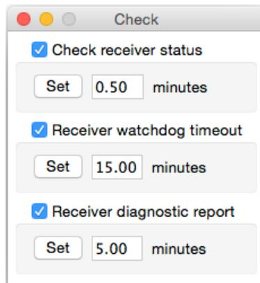
The Watchdog Control window allows you to change how often SeaSondeController checks the receiver's settings, change the receiver's watchdog time out value, and change how often for SeaSondeController to write out new entries into the hardware diagnostics file.
