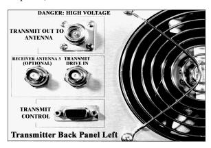
Connect an **RG-8** cable between "**Transmit out to Antenna**" to the Transmit Antenna. There is an **electrical junction box** at the **base** of the Transmit Antenna, where a connection can be made:
