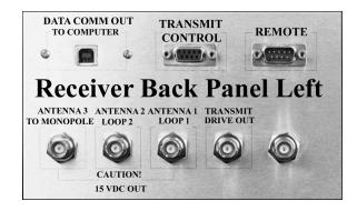
Connections from the Receiver go to the Receive Antenna. At the **base** of the Receive Antenna, you will find connectors **arranged like these**:
